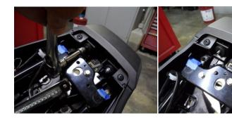
5. Install the supplied DMP base plate. Make sure the front of the base plate slides into the two slots on the undertail as well as clearing the center piece. Bolt the base plate to the bike using two of the 8x20 bolts with four of the 8mm washers and two of the 8mm lock nuts toward the front of the base plate.
