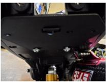
6. Install the DMP license plate bracket using two of the 8x20 bolts with four of the 8mm washers and two of the 8mm lock nuts and remount the brake light.
