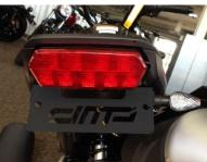
7. Mount supplied DMP market lights (900-0070). Be careful not to over tighten the market light nuts. Route the OEM turn signal wire harness and plug it in (step 2 in reverse). Plug in the DMP turn signal wires to the previously identified left and right wires from step 2. The Yellow marker light wire is the Positive lead and Negative is Black.
