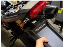
4. Remove the stock tail light by removing the two lock nuts holding it into place.
