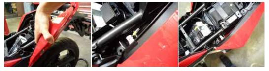
7. Un plug the brake light and remove the tail section. Double check to make sure that all the tail section bolts and rivets have been removed. Stand behind the bike, lightly spread and pull the
