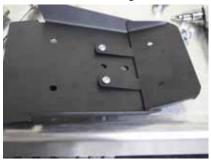
12. Attach the plate bracket to the back plate using two 6x1.00x12 button head bolts, four 6x15 (larger 6mm) washers and two 6x1.00 lock nuts.
