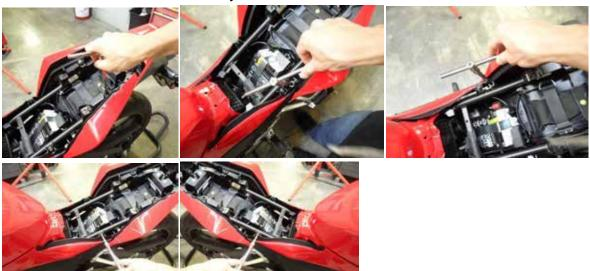
6. Remove the key cable. Lightly pull the left side tail section away from the sub frame and unhook the cable.
