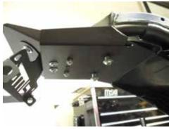
14. Loosely mount the two L tabs with the rubber grommets to the 8x25mm bolts using two 8mm washers and locknuts. Using the proper size wrench, while holding one tab with one hand (make sure tab is facing the correct direction as shown below) tighten the nut until you can barely turn the tab by hand. Repeat on opposite tab.
