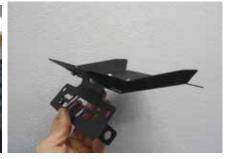
13. Mount the DMP Fender Kit to the back of the motorcycle using two 8x1.25x25 with 8mm washers and two 6x1.0x12 with 6mm fender (large) washers. We recommend using medium thread locker on the 6mm bolts.
