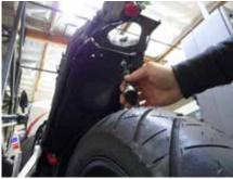
11. Assemble the center plate with the back plate using two 6x1.00x12 button head bolts passing through the top (make sure the button head bolts are used as pictured below for proper clearance) and from underneath use two supplied 6x15 (larger 6mm) washers and two 6x1.00 lock nuts. Tighten the hardware.
