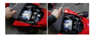
6. Remove the key cable. Lightly pull the left side tail section away from the sub frame and unhook the cable.
