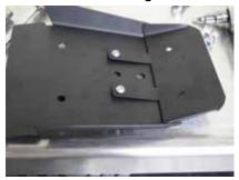
12. Attach the plate bracket to the back plate using two 6x1.00x12 button head bolts, four 6x15 (larger 6mm) washers and two 6x1.00 lock nuts.
