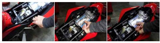
7. Un plug the brake light and remove the tail section. Double check to make sure that all the tail section bolts and rivets have been removed. Stand behind the bike, lightly spread and pull the tail section body work toward you. The tail section will be hard to remove until the tail light pulls from the rubber grommets.
