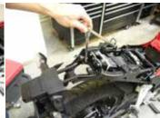
9. Remove the rubber grommets on the stock fender (pay attention to the way the grommets are facing) and install them on the two L brackets provided by DMP. Make sure the rubber grommets are facing the correct way for install.
