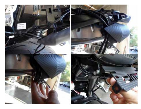
20. Install tail section and seats. Make sure all bolts are tightened to the proper torque specifications.
