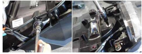
9. Slide the flashing cover (with the DMP bracket mounted) onto the rear exhaust cover. Make sure the slot on the flashing cover slides onto the rear pipe cover track.
