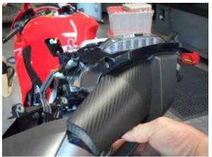
5. Separate the OEM fender and remove the stock pipe flashing covers.
