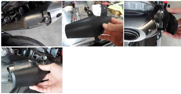
10. On the right hand side, line the rear hole of the DMP fender bracket with the rear hole on the sub frame and install the 6x16 bolt with the 6x15 (larger 6mm washer) washer. Keep the bolt loose.
