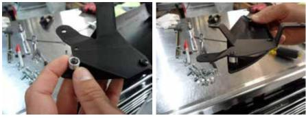
7. Install the rear pipe cover but leave the bolts loose.
