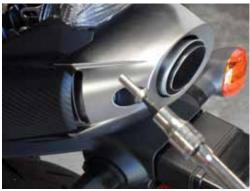
8. Remove exhaust sub frame and alignment bolt (alignment bolt is located in front of the brake light).
