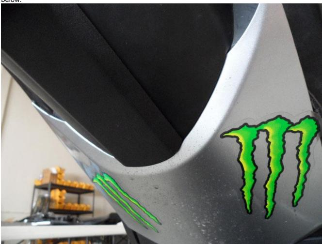
7. Reinstall fender. The seam of the bottom support plate should like up with the bodywork as shown below.
