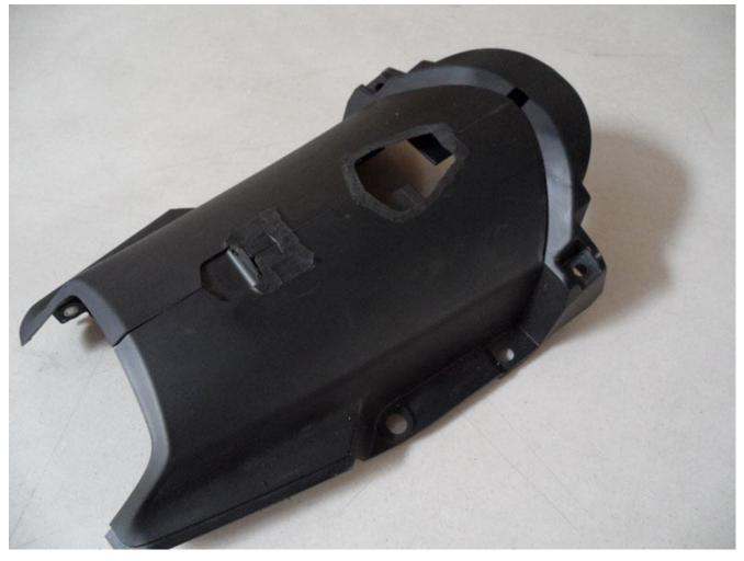
4. MAKE SURE YOU HAVE SAFETY GOGGLES AND GLOVES ON DURING THIS PROCESS! In this section of the install we had to make a provision for a wiring harness. We simply took a Dremel and sanding roll to make a clearance notch.
