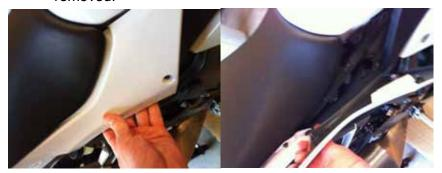
6. Remove the forward seat bolts on the left and right hand side. Remove the seat.
