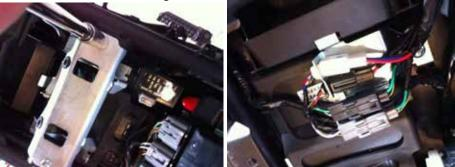
10. Unclip each connection (It is recommended that you identify each connection and mark them before being removed)
