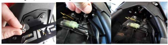
20. Pull slack from wires through the tail section and snap the OEM cap that was removed earlier back into place
