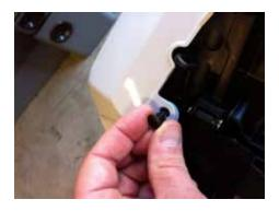
5. Remove side panel. Bodywork is snapped into place, be careful removing the body work, do not force. If you are having issues double check to make sure all bolts and rivets have been removed.
