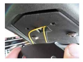
19. Using the larger 6mm washer and 6x16mm bolt insert into the open hole. On the inside of the tail section slide the larger 6mm washer over the bolt and screw on the 6mm lock nut. Using a socket wrench on one side and an allen wrench on the other torque down the bolts. Do not over tighten, the lock nuts have nylon to keep from coming loose.
