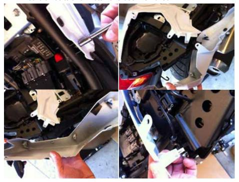
9. Remove tail section wiring harness cover and expose the connectors
