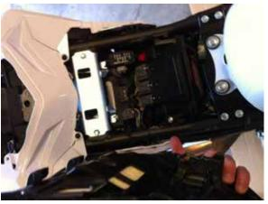
7. Remove tail section Rivets
