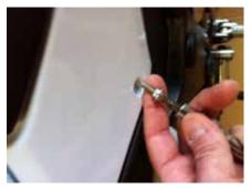
4. Remove body work rivets
