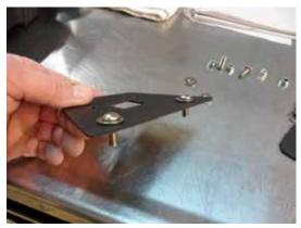
17. Holding the bolts in place flip the bracket upside down and place through the fender holes underneath the tail section. Place the larger 6mm washers over the bolts on the inside and screw on the lock nuts. Using a socket wrench on one side and an allen wrench on the other torque down the bolts. Do not over tighten, the lock nuts have nylon to keep from coming loose.
