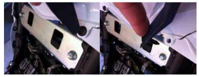
8. Remove tail section side bolts and remove tail section. Bodywork is snapped into place, be careful removing the body work, do not force. If you are having issues double check to make sure all bolts and rivets have been removed.
