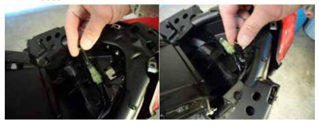
18. Line the bottom plate up with two open holes of the plate that was just installed (the wires shown in this picture are from the DMP marker lights installed to the fender plate)
