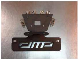
16. Take two of the 6x16mm bolts and 2 of the larger 6mm washers and place it through the plate shown below
