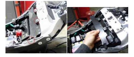
4. Remove the turn signal housing that holds the turn signal connectors in place. Identify and mark the left and right hand turn signals. Disconnect the turn signal and plate light connections.
