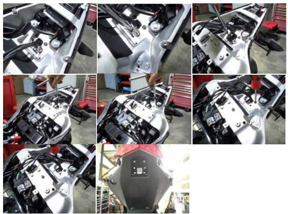
6. Mount the DMP base plate using two 6x1.0x20 bolts, four 6x15 (larger) washers and two 6x1.0 lock nuts.
