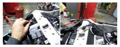
5. Remove the fender by removing the four fender button head bolts and the two philip head screws holding the fender in place. Guide the wires through the center hole.
