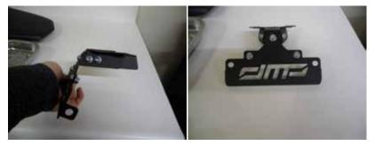
8. Mount the DMP Fender Kit using the 4 x 6x1.0x16 bolts, 4 x 6x15 (larger) washers and 4 x 6x1.0 lock nuts.
