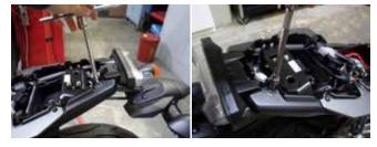
4. Remove the rear seat bracket by removing these four bolts.
