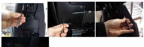
3. Remove the tail section bolts shown below to expose the rear seat bracket bolts.
