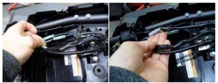
6. Remove the stock fender by removing the final four nuts holding it in place.
