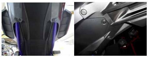
3. Remove forward tail section screws.
