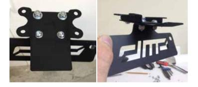
10. Bolt the assembled DMP Fender Kit to the bike using four 6x1.0x12 button bolts and four 6x15 (larger) washers. Make sure you use medium thread locker on each bolt.
