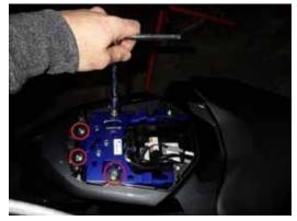
6. Locate, cut and remove the wiring zip tie. Unsnap the wiring clamp.
