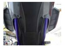
12. There are three rivets left, two larger rivets and one smaller rivet. Apply the two larger supplied plastic spacers to the larger rivets and the smaller spacer to the smaller rivet. Press the rivets back into place as shown. This will allow for a clean look without having to worry about the rivets falling out of place.
