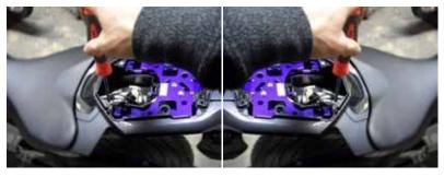
4. Remove rear tail section screws and tail light bodywork cover. Slide the cover back toward the rear of the bike.
