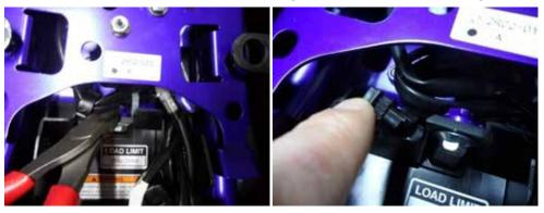
7. Locate the turn signal and plate light connections and un plug them. Make sure you identify and mark the left and right hand turn signals before unplugging them.
