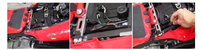
6. Remove two front OEM fender nuts (the back nut will hold the fender in place). Remove the rear bolt and nut (you may need assistance). While removing the OEM fender feed the plate light through the plate light hole.
