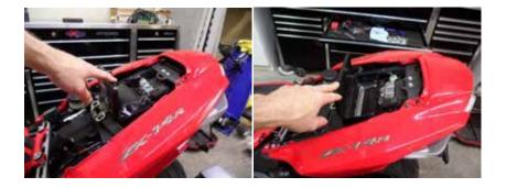
3. Remove the connector and foam housing to the left of the wire harness (left side facing the rear of the bike). Don't unplug the connector.
