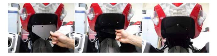
In the same sequence as step 7, install the DMP bracket using the two 6x1.00x16 bolts, two 6x15 washers, two 6x12 washers and two 6x1.00 lock nuts. Make sure all hardware is properly tightened.
