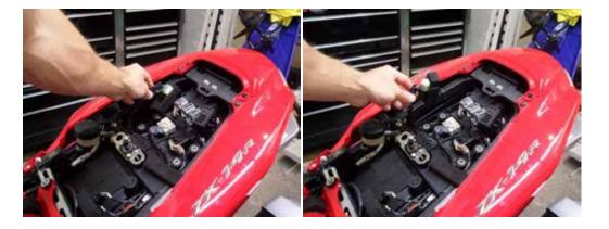
4. Remove the rubber wire harness. The wire harness has two hooks holding it in place (one on each side). Manipulate the rubber and slide the harness up and out of the way.
