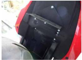
9. The remaining DMP hardware is used for mounting the license plate.
