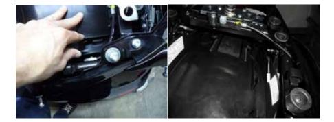
There is a zip tie that holds the wires to the frame on the left hand side. You will need to loosen the undertail in order to cut the zip tie to remove the fender. Follow these steps in order to complete the fender eliminator process.
