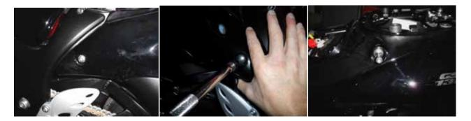
4. Remove the plastic undertail fender rivets on the left hand side.
