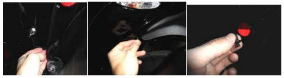
11. Install the left side body panel bolts. Use a flash light to help line up the holes.
