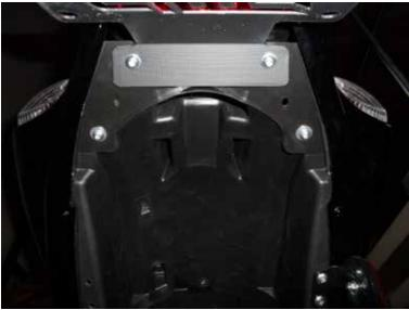
9. Re install the undertail bracket. Install the left bolt first (left bolt is more open and easier to access). Use a flash light for assistance.
