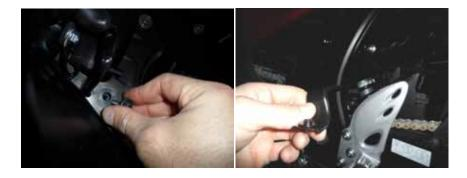
6. Remove the four bolts holding the stock fender in place. (the fender will not be able to be removed until the zip tie has been accessed and cut)
