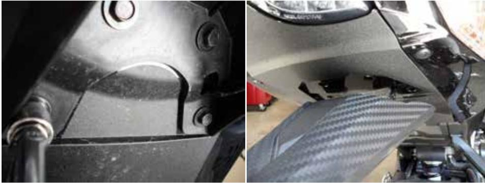
4- Locate the plate light from inside the tail section. Remove the stock fender and tail section body work. Unplug the plate light connection. Fender should come right off.
