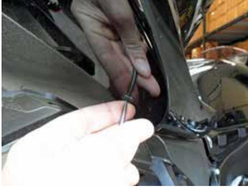
3 – Remove the four fender bolts from underneath the tail section.
