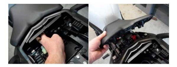
2. Un bolt the four bolts that are holding the OEM fender in place.
