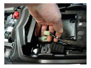
5. Remove the wire covers and un plug the turn signal and plate light connections. Make sure you identify and mark off the left and right turn signals as well as the plate light positive and negative.
