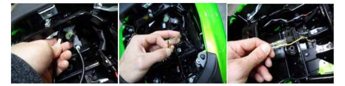
13. Mount your license plate using the two DMP plate lights (900-2042) and hardware. Feed the wires through the center hole of the DMP fender eliminator. We prefer to use the stock plate light connector and wires. Cut the OEM plate light wires to length one at a time. Crimp the butt connectors supplied and pull on each wire to make sure there is a solid connection.
