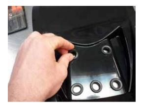
9. Remount the entire tail section and fender following step 6 in reverse. Make sure the fender rivets are put in place and the tail light is plugged in.
