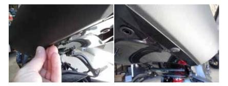
10. Loosely mount the DMP fender kit using the four 8x1.25x30 mm bolts, eight 8mm washers and four 8mm lock nuts. Once the plate is loosely mounted, tighten the plate caddy corner until it's tight. (remaining hardware is for mounting the license plate)
