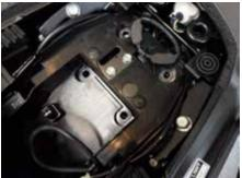
3. Remove the body rivets located from underneath the tail section.
