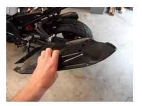
8. Add the 5 rubber grommets to the fender as shown below.
