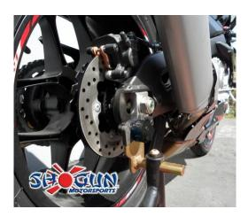
WARNING: DO NOT MOUNT THE SPOOLS TO THE FORWARD SWING ARM LUG. THE CLEARANCE TO THE EXHAUST MAY NOT BE ENOUGH.
