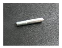
With the body removed, thread the spot tool into engine mount location. Make sure you have the spot tool screwed in enough to clear the body on the inside.
