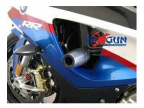
2. Remove left side bolt. Mount right side puck with (99-HB-SH1015090) Socket Cap 10 X 1.5 X 90 Main Engine Stud and torque down to the recommended OEM torque specifications.
