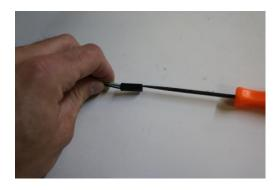
3. Install the Yellow wire (Right Positive lead) into the Black plastic housing. Make sure the connector is facing right side up from top to bottom and inserted into the previously identified positive side. If the wire is put in upside down, the connector will be pushed out when pressed into the harness. Repeat with the Blue wire and Grey OEM plastic housing. Note: In our example we are using two black OEM plastic housings.
