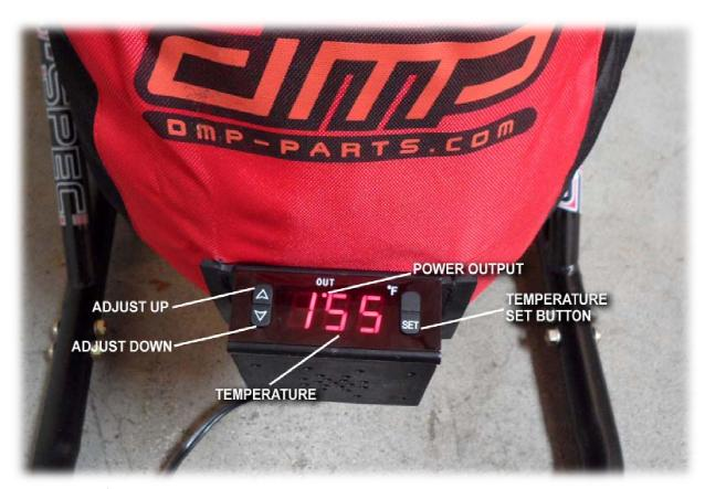
Install front and rear tire warmers using high strength Velcro straps supplied on the warmer by carefully pulling the warmer element over the tire. Tires <u>must</u> be properly elevated using front and rear stands. Bunching, overlapping, or folding over heated areas of the warmer may cause overheating and damage the warmer!
