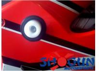
10. Remove left side bolt. Mount left side puck with (99-HB-SH101250100) Socket Cap 10 X 1.25 X 100 Main Engine Stud and torque down.
