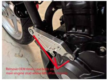
3. Before left side offset is installed pre assemble the offset using two 6 X 1.00 X 60 (99-HB-SH0610060) socket cap bolts and two 25mm offset spacers (428-9108) with the larger diameter part of the spacer towards the backside of the offset.
