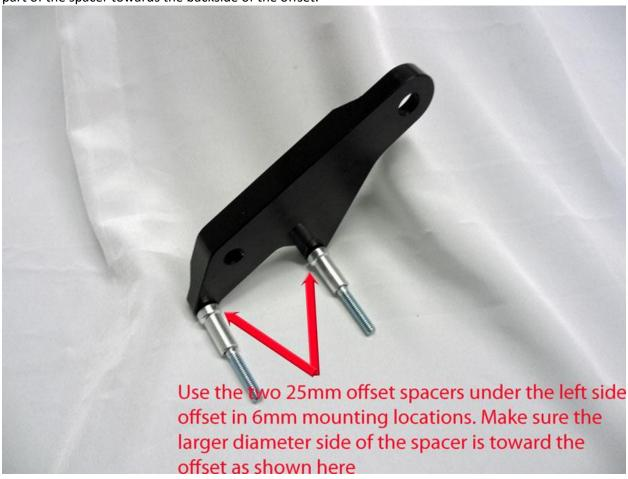
4. Mount left side offset (LOOSELY) by hand using all 3 bolts. Tighten both 6 X 1.00 X 60 (99-HB-SH0610060) socket cap bolts (FIRST) then main OEM engine stud. Check service manual for 6mm and main engine stud OEM torque specs.
