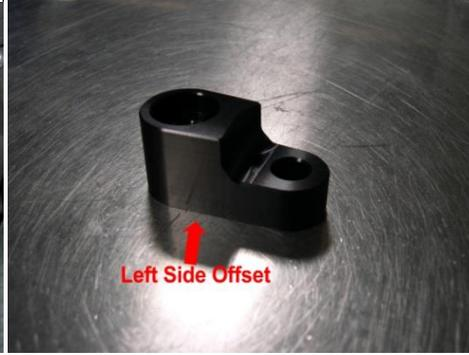
3. Mount the left side offset using the stock OEM 12mm Hex Flange bolt. Make sure that the wire loom is routed properly and not being pinched by the offset in anyway. Line up the edge of the offset (wile mounted) with the edge of the frame and torque down.
