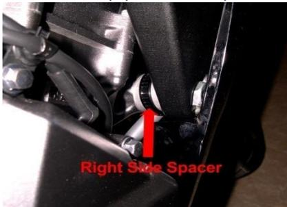
6. Mount the right side offset using the stock OEM 12mm Hex Flange bolt. Make sure that the wire loom is routed properly and not being pinched by the offset in anyway. Line up the edge of the offset (wile mounted) with the edge of the frame and torque down.
