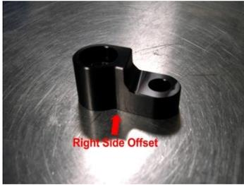
7. Use one drop of blue thread locker on the (99-HB-SH10125070) Socket Cap 10 X 1.25 X 70 (Holds puck to offset). Torque down to 30 to 32 foot lbs.
