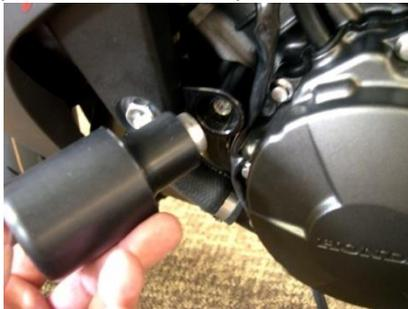
5. Remove right engine stud. There is a spacer that is located between the frame and the engine. Your right side offset will mount in this location. The zip tie located around the spacer is reusable, simply unlock it by hand so you can reuse later.
