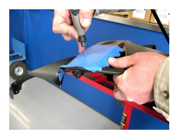
6. Using a small drill 1/8 inch or so drill a pilot hole in the body(see above photo). Remount bodywork and double check the hole location with the spot tool still inserted (arrow in picture below is pointing to spot tool). With pilot hole cut and on center, remove body panel to prep for cutting.
