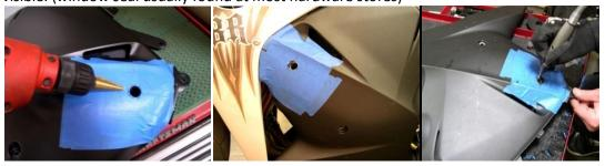
9. Mount body then slider then torque down to OEM specs. Remember each side was done the same way.
