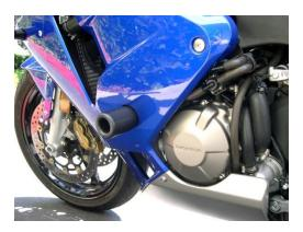
10. Remove right side bolt. Mount right side puck with (99-HB-SH121250120) Socket Cap 12 X 1.25 X 120 Main Engine Stud and torque down.
