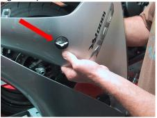
11. Remove right side bolt. Mount right side puck with (99-HB-SH12125090) Socket Cap 12 X 1.25 X 90 Main Engine Stud and torque down.
