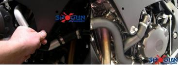
6. Remove the bodywork and double check location of spot mark the tool has created.
