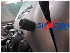
12. Remove left side bolt. Mount left side puck with (99-HB-SH12125090) Socket Cap 12 X 1.25 X 90 Main Engine Stud and torque down.
