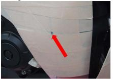
8. A pencil was then used to draw our diameter of desired shaped hole. A flexible hole template can also be used for the same purpose. Place the hole template on center of the pilot hole (or spot tool) and draw your desired diameter.
