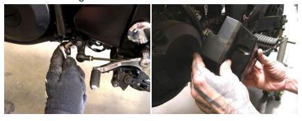
4. Loosen front and rear engine through studs. Do not remove studs until after step 5.
