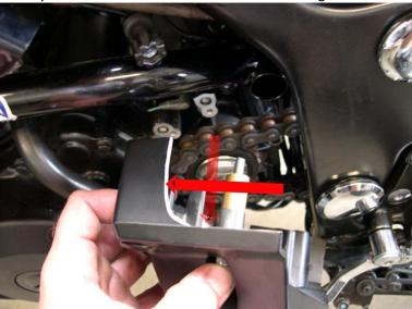
This cut out is clearance for the rear of the left rail.
