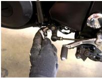
12. Mount left and right side sliders using 99-HB-SH10125080 Socket Cap 10 X 1.25 X 80 (Holds puck to offset) 99-HW-M10WASH Washer M10 Zinc Plated 99-LN-LN10125 (one washer goes under the head of the bolt, one goes under the Hex Lock Nut) Hex Lock Nut 10 X 1.25 (Left side slider longer than right)Torque down to 40 ft lbs.
