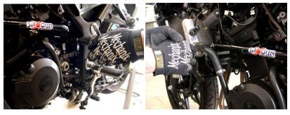
7. Mount the right side rail using(99-HN-LN9/1618-F&R) 9/16 18 Pitch Hex Flange Serrated Nuts and torque down to 32ft lbs.
