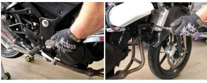
8. Counter Shaft Cover Prep: Use several layers of masking tape to completely mask off the area on the cover where you will be working. Tape the area where you will cut and also the sides of the part so when you hold it with another device (such as a vise or table clamp) it doesn't damage or
