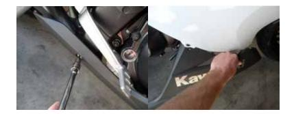
5. Remove inner radiator cowl. Note: To remove body clips press the center inward to release plastic rivet. There are also two bolts that need to be removed located directly in front of the radiator.
