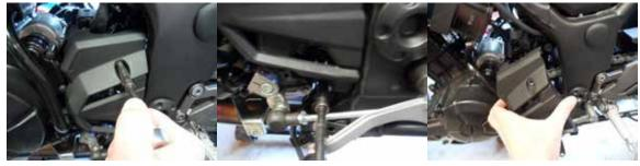
9. Make sure the vehicle is in a fixed secure position. With a standard floor jack support the engine enough to remove engine studs. To help prevent scratching of any kind or damage to the bike when lifting we use a small piece of soft wood or a plastic puck on the jack pad. With jack secure and in place remove each front and rear stock engine studs.
