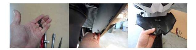
6. Remove the two left and right body screws located underneath the head light assembly.
