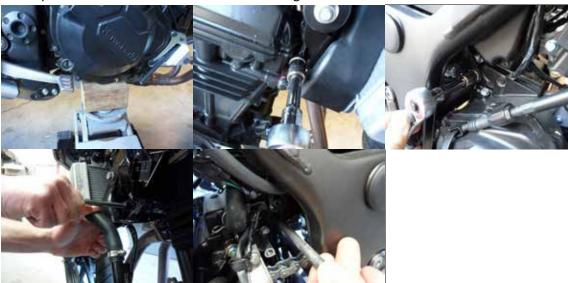
10. Remove left side harness bracket. Note: The rubber coated connector has to be unplugged to be removed from bracket the other unclips from the bracket.
