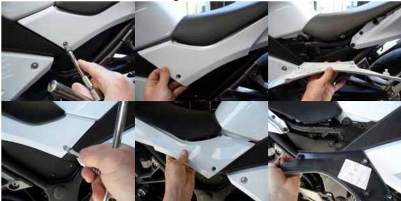
3. Remove upper mid panels left and right located under the gas tank.
