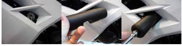
16. Mount right side puck using 10 X 1.5 X 90 (99-HB-SH10150090)bolt and washer. There is a cutout in the puck to clear the body orientate the puck and torque down to 35ft lbs.
