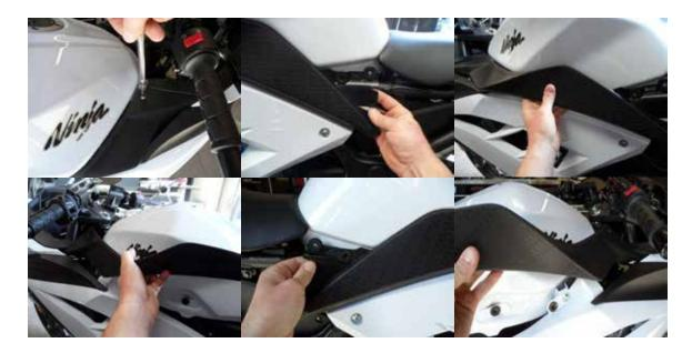
4. Remove lower body cowls left and right. Note: To remove plastic body clips use a flathead screwdriver and lightly pop out the center of clip.
