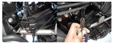
13. Loosely mount the counter shaft sprocket cover to create a clearance pattern. Once you have created clearance for the left side rail mount the counter shaft cover and tighten up.
