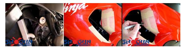
7. Using a sharpie pen we make a point where the center of the engine stud would be. (picture 3<sup>rd</sup> to the right shown above)
