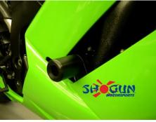
5. Put one drop of blue thread locker on the end of the thread mount right side puck to the offset using 99-HB-SH10150045 Socket Cap 10 X 1.5 X 45. Torque down to 30 to 32 foot lbs.
