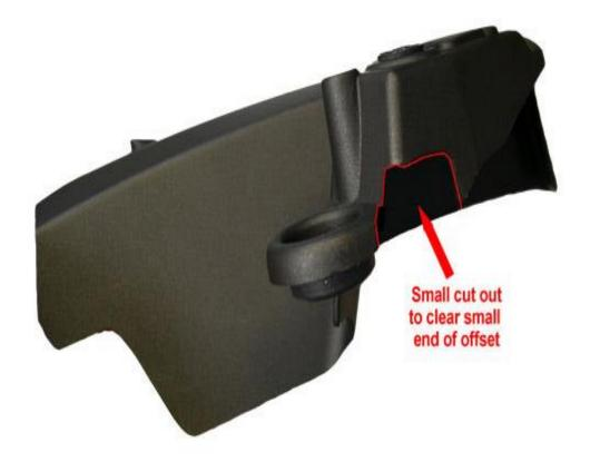
2. Once you have notched the small left side panel, mount the left side offset but only hand tight. You need to be able to move the offset by hand to its proper location.
