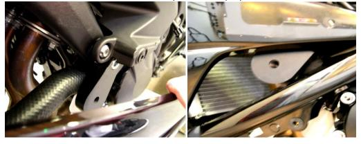
3. Mount the left side bodywork and align the offset to the opening in the body. Mount the left side slider on the offset to ensure correct location. There is a flat notch in the slider so the body will clear. Remove the slider and body and torque down the offset to OEM specifications. (see above)
