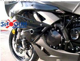
5. Mount right side offset using (10 X 1.25 X 70) make sure you can still move the offset by hand. Mount the body loosely and angle the offset to the opening in the body. Make sure that the slider clears the body and mounts clean to the offset. Remove the slider and body and torque down the offset to the OEM specifications.
