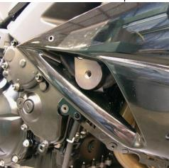
6. Mount the right side panel. Install the slider using one drop of blue thread locker and torque down to 30 to 32 ft lbs.
