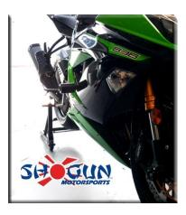
2. Remove left side bolt. Mount left side puck and spacer (longer puck with longer spacer) with (99-HB-SH10125110) Socket Cap 10 X 1.25 X 110 Main Engine Stud and torque down to OEM torque specifications.
