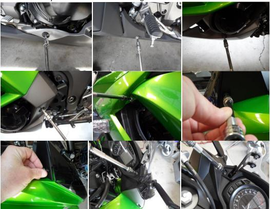
Start by removing the lower cowling first (Note: If you have any issues removing the body work, double check to make sure all rivets and bolts have been removed)
