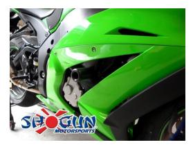
2. Remove Left side engine stud and mount Left side frame slider using 99-HB-SH1012590 Socket Cap 10 X 1.25 X 90 Main Engine Stud and torque down to OEM torque specs.
