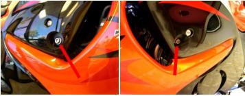
9. Remove right side bolt. Mount right side puck with (99-HB-SH10125100) Socket Cap 10 X 1.25 X 100 Main Engine Stud and torque down.
