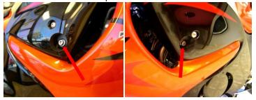
Remove right side bolt. Mount right side puck with (99-HB-SH10125090) Socket Cap 10 X 1.25 X 90 Main Engine Stud and torque down.
