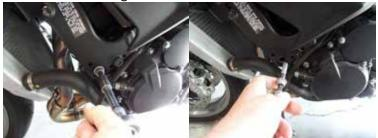
4. Mount left side offset to the motorcycle. Read your service manual for specific torque specifications associated to those locations. Use (99-HB-SH10125060) 10 X 1.25 X 60 Socket cap bolt with 10mm steel washer to mount offset to the motorcycle. Torque down main engine stud. Tip: DO NOT use blue thread locker on either bolts discussed in this section. Start bolt in by hand make sure you have good thread engagement do not cross thread.
