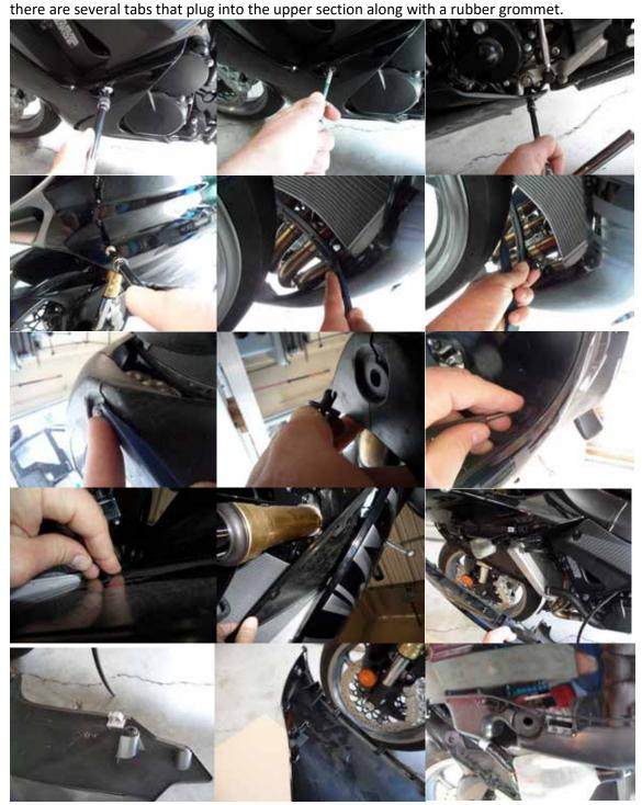
2. Attach the threaded frame cup spacers (99-SP-750-5410-L&R) to both left (99-OF-750-5450-L) and right (99-OF-750-5450-R) offsets using one drop of blue thread locker on the end of the 8mm (99-HB-0812520) socket cap button head bolts. Tip: Do not attach frame slider pucks.
