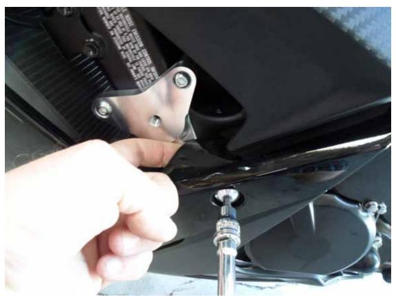
9. Mount frame sliders left and right to the offsets. Left side frame slider is longer than right. Use (99-HB-SH10150035) 10 X 1.5 X 35 Socket cap bolts with one drop of blue thread locker on each bolt and torque down to 32 foot lbs.
