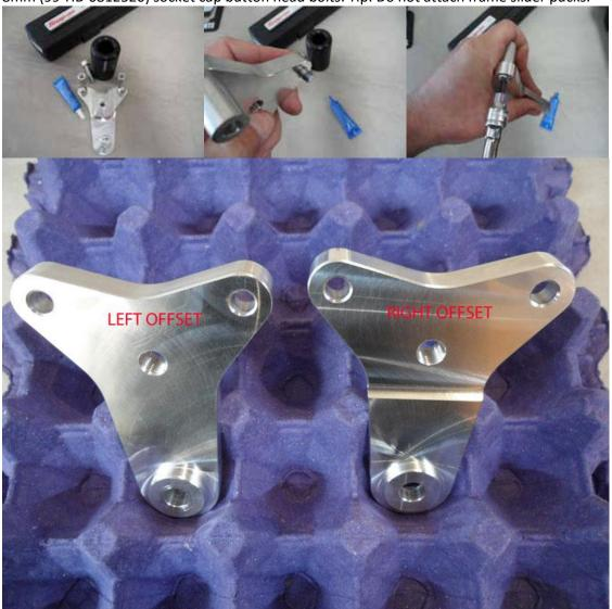
The photo above shows the back side of the offset (the side that will be facing the frame) you can see the right side offset has a radius step. This is so the offset will clear VIN tag on the right side of the frame.
