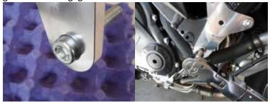
8. Mount bodywork. On the left side you will need to guide the body panel up the offset as you tighten body screw shown in this photo. This Shogun kit has a very tight fit on both the left and right side this is to ensure the maximum strength of the offsets.
