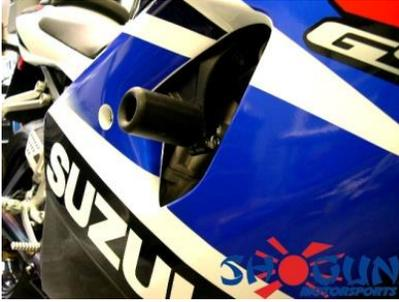
3. Remove left side panel. Remove left engine stud. Use 99-HB-SH10125070 Socket Cap 10 X 1.25 X 70 (Goes through the Offset into the Frame) Main Engine Stud. Make sure your offset is at the correct angle so the puck will clear the body. Torque down to OEM torque specs.
