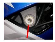
2. Use the (99-HB-SH10125090) Socket Cap 10 X 1.25 X 90 Main Engine Stud to mount the Right side frame slider. There is a notch cut in the right side frame slider (arrow is pointing to notch and crush spacer) this notch is so the body will clear the slider. Torque down to OEM torque specs.
