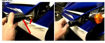
3. Remove left side panel. Remove left engine stud. Use 99-HB-SH10125070 Socket Cap 10 X 1.25 X 70 (Goes Though the Offset into the Frame) Main Engine Stud. Make sure your offset is at the correct angle so the puck will clear the body. Torque down to OEM torque specs.
