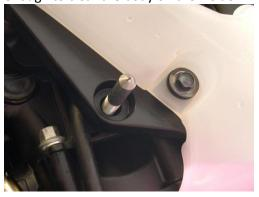
5. Loosely mount your bodywork and adjust the spot tool out to lightly touch the inside of the body. Make sure you have at least 15mm of thread engagement, without that the spot tool will tend to sag down giving you a false location. With the body mounted in the correct location use a soft micro fiber cloth over the spot tool location and softly tap to leave a spot mark on the inside of the body. Be careful not to scratch or chip the body.
