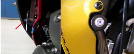
2. Locate the left side engine stud and remove bolt. Make sure the conical spacers stay in frame when frame sliders are installed.
