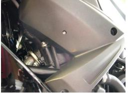
8. Body Prep. Use masking tape to completely mask off the area on the body where you will be working. We usually will tape off approximately 6 to 8 inches around the though hole area and any other edges that could get bumped or scratched while working. Tip: In some locations you may want to double up the thickness of the masking take to give extra protection.
