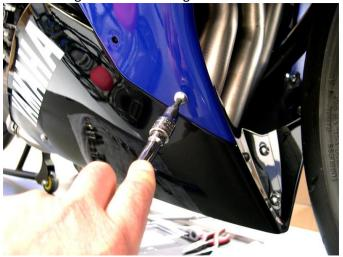
2. Remove the left side engine stud. Mount the left side offset using 99-HB-SH12125090 Socket Cap 12 X 1.25 X 90 Main Engine Stud and torque down to OEM torque specs.
