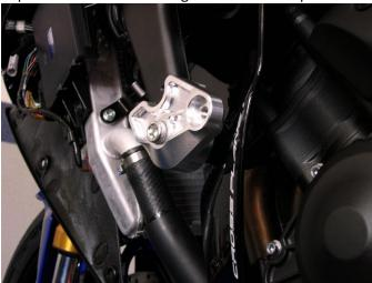
3. Using one drop of blue thread locker mount the left side puck to the offset with 99-HB-SH10125060 Socket Cap 10 X 1.25 X 60 (Holds puck to offset). Torque down to 33 to 35 foot lbs.
