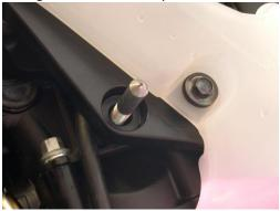
5. Loosely mount your bodywork and adjust the spot tool out to lightly touch the inside of the body. Make sure you have at least 15mm of thread engagement, without that the spot tool will tend to sag down giving you a false location. With the body mounted in the correct location use a soft micro fiber cloth over the spot tool location and softly tap to leave a spot mark on the inside of the body. Be careful not to scratch or chip the body.
