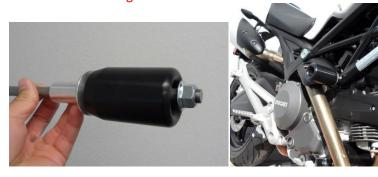
4. Install left spacer (428-9110) and left hand slider (99-FS-750-8209-L) with provided nut (99-HN-LN12125). Torque nut down to the OEM torque specifications.
