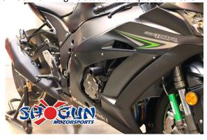
2. Remove Left side engine stud and mount Left side frame slider using 99-HB-SH1012590 Socket Cap 10 X 1.25 X 90 Main Engine Stud and torque down to OEM torque specs.
