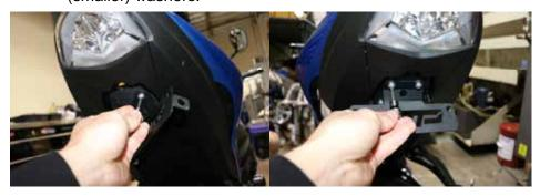
11. Install the desired turn signals and plate lights. We recommend using DMP turn signals to complete the install.
