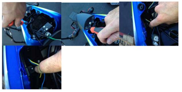
5. Remove the right side tail section by un snapping and sliding the tail section bodywork toward the front of the bike.
