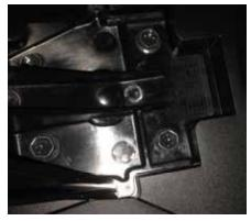
9. Mount the DMP base plate using the two supplied 6x1.0x12 button head bolts and two 6x12 (smaller) washers. Use medium thread locker on these bolts.
