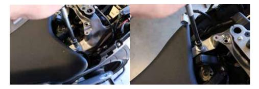
6. Identify and unplug the left and right hand turn signal connections. Unplug the plate light connection.
