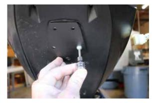
10. Mount the DMP license plate bracket using the two 6x1.0x16 bolts with two 6x12 (smaller) washers (medium thread locker is recommended).
