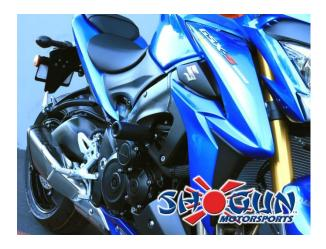
2. Remove left side bolt. Mount left side puck with (99-HB-SH10125080) Socket Cap 10 X 1.25 X 80 Main Engine Stud and torque down to the recommend OEM torque specifications.
