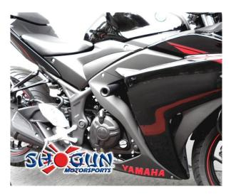
2. Remove the right side bolt. Mount the right side puck with (99-HB-SH10125100) Socket Cap 10 X 1.25 X 100 Main Engine Stud and torque down to the recommended OEM torque specifications.
