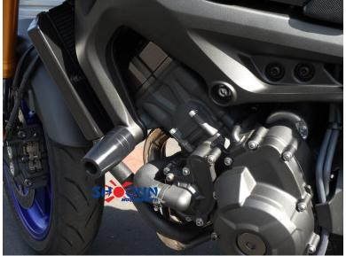
2. Remove right side bolt. Mount right side puck with (99-HB-SH10125080) Socket Cap 10 X 1.25 X 80 Main Engine Stud and torque down.
